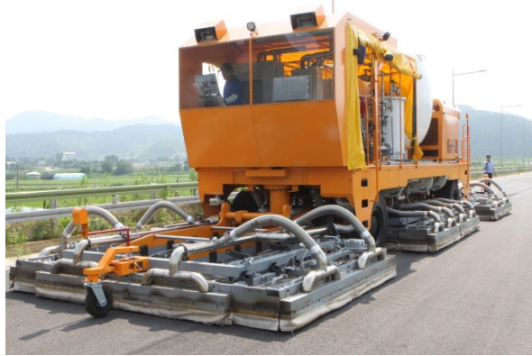
Figure 2-10 Emission controlled heating equipment for asphalt pavement recycling
